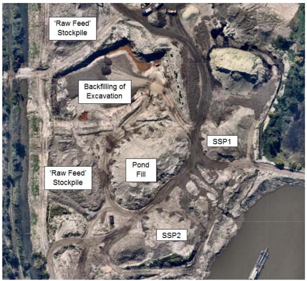
Figure 1: Aerial photograph showing SSP1, SSP2, 'pond fill', 'raw feed' stockpiles and the excavation (Source, NearMap flown 9 September 2016)
